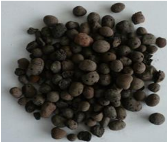
Argex, \rho_{rd} = \pm 1100 \text{ kg/m}^3
